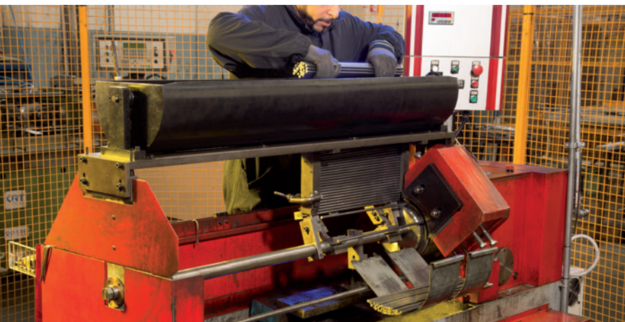
Automatic threading performed with the rotary rolling process
