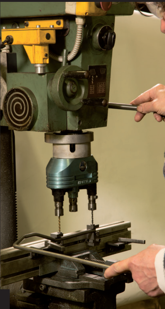
Multiple drilling operations on already bent parts
