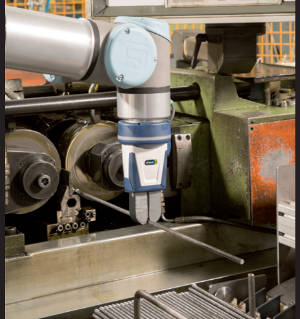
Threading performed with the rolling process with robotized loading and unloading
