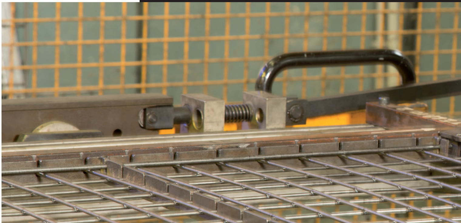
Three-dimensional system for medium frequency welding with 8-axis CNC movement
