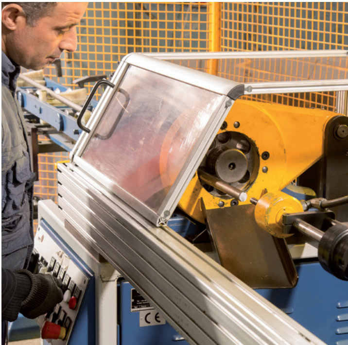
Semi-automatic cutting of bars up to Ø30
