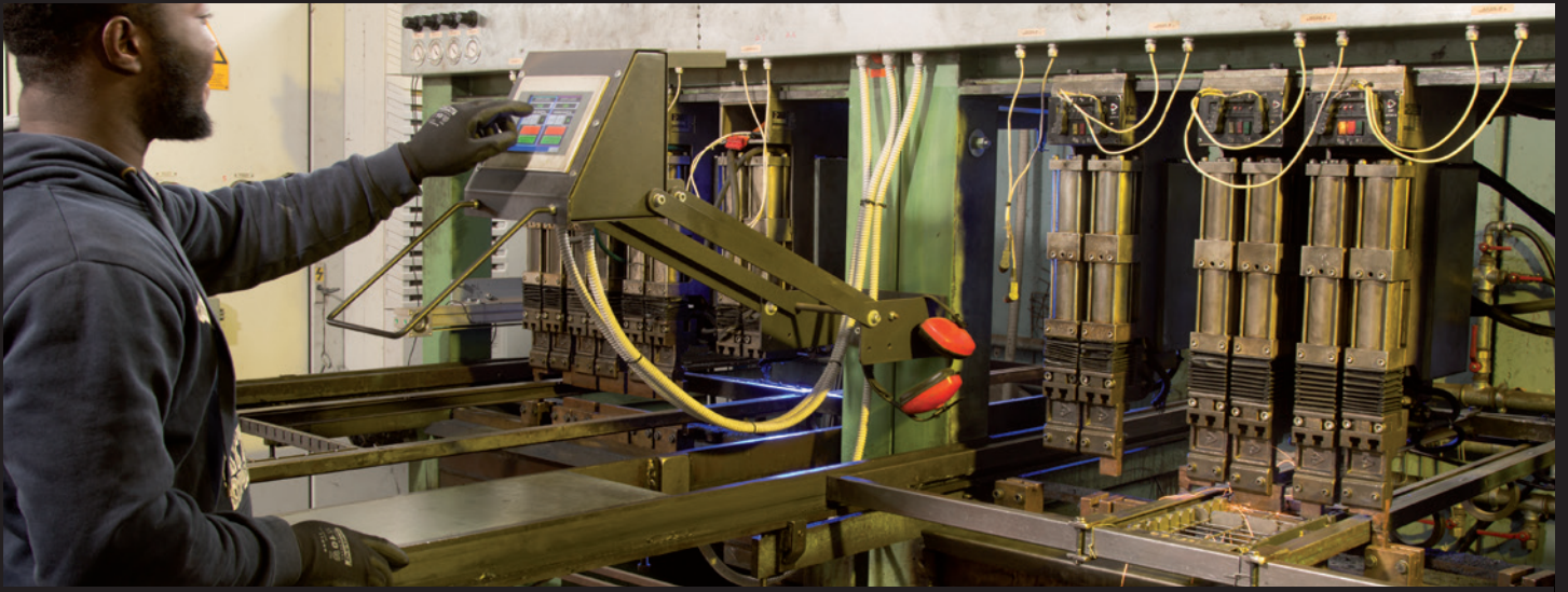
Resistance welding with semi-automatic cycle
